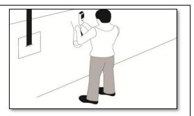
5.8.3. When carrying-out a CO<sub>2</sub> treatment, the approximate CO<sub>2</sub> concentrations can be determined by measuring CO<sub>2</sub> concentrations using the carbon dioxide analyzer.
