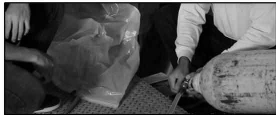
4.3.7.2. Flushing (emptying of the cylinder) depends on the amount of CO<sub>2</sub> to be applied. Emptying one 22kg cylinder should only take about 20 to 30 minutes. If the pressure hose or the inlet valve gets blocked with ice, this is an indication that the CO<sub>2</sub> is being released too quickly. If this happens the cylinder should be closed until the ice melts, and then the cylinder valve should be re-opened and adjusted to reduce the flow.
