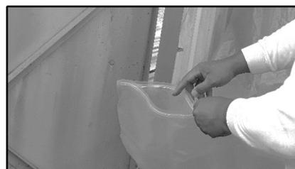
4.3.6. Open the cylinder valve. Adjust opening of the valve until sound of liquid passing through the hose is heard. The liquid CO<sub>2</sub> flushes into the TSL and evaporates inside, it pushes the air upward, acting as a piston, until the air is totally replaced. The opening through the zipper serve as an outlet for the displaced air.
