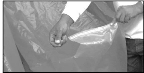
3.3.4. Position the zipper slider on the manually zipped portion of the zip lock.
