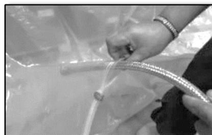
4.3.5. Open a section of the zipper and insert the pressure kit. This serves as outlet to discharge O<sub>2</sub> when flushing.
