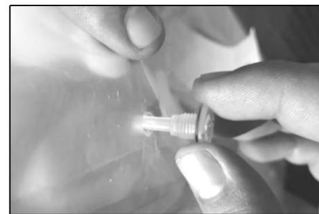
3.2.4. Screw the plastic valve body. The cap of the plastic valve should be positioned outside the loaded TSL. Firmly tightened the body into the base to prevent leakage.
