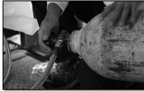
4.3.7. Ice formation along the pressurized hose and the pipe connector during CO<sub>2</sub> flushing:
