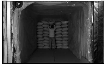
2.1.5. When stacking bags, make sure to leave at least 20cm distance between the roof of the container and top of the stacks to prevent condensation.
