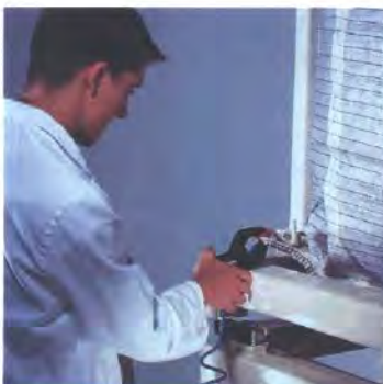
Earthing clamp is fixed to loop of Type C bag.
