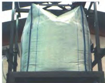
Pneumatic side massagers are adjustable in height depending on the product flow properties and bulk density.
