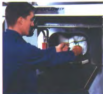
Access door allows untying of bag tie string.
