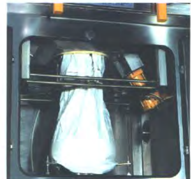
Inflatable spout sealing and stretching device (Patented)
