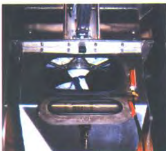
Yoke type spout closure bars (patented).
