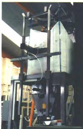
2. Bag is lifted by FLT on to discharger and kept under tension with spring loaded side support arms.
