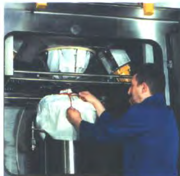
Spout closure bars close off bag whilst operator places spout over seal and unifies the bag.
