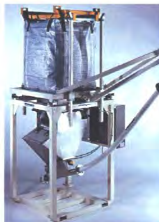
Earthing clamp is fixed to loop of Type C bag.
