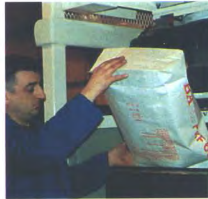
Sack dump door in discharger base.
