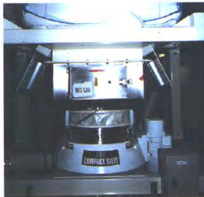
Integral sieve fitted to discharge chute.
