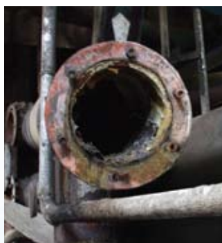
Metal pipe shown here exhibiting both internal and external corrosion.
