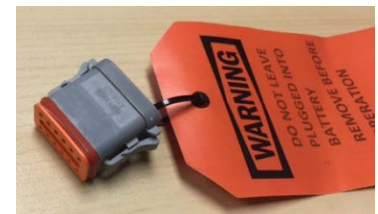
Figure 4: A Jumper Plug. It is used to revive an over-discharged LiFT Pack.
