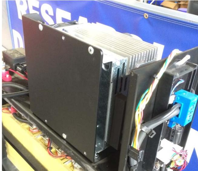
Figure 5: The charger mount and rivets.
