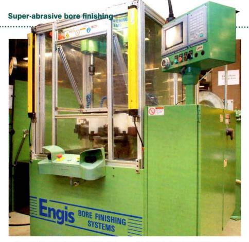
Bore roundness also features a critical tolerance, while bore surface finish is a further strict requirement. All of these production challenges are now described as "no problem whatsoever", using the Engis machine. The four spindles of the machine are tooled to produce a sequence of: rough; semi-rough; brush; and finish. Programming the machine's Mitsubishi CNC is extremely simple, and all spindles come down simultaneously, with the
