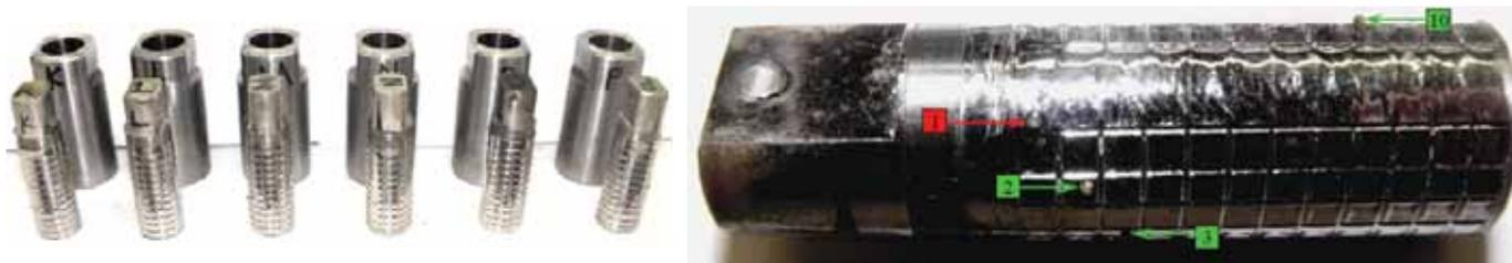
Fig 24 Actual diamond electroplated rods and respective cylinders
