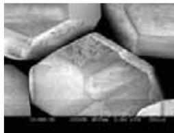
Fig 6f SEM micrograph of heavily etched 40/50 mesh saw grade diamond particles (250X magnification)
