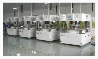
Features include, automatic slurry delivery, variable in cycle pneumatic pressure control and plate temperature control.
