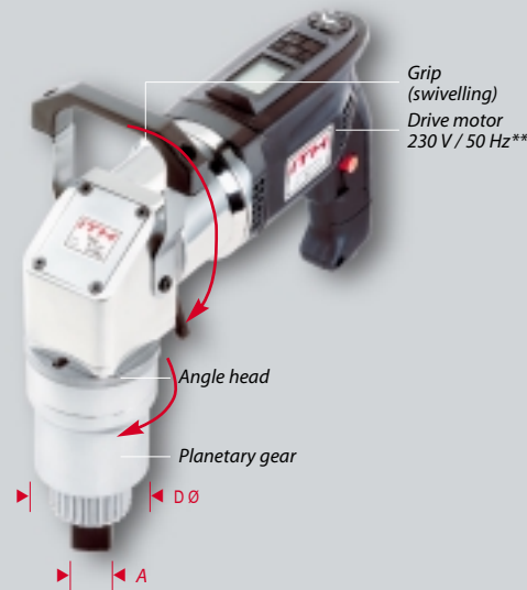
Type EDSw*- \alpha Rotation-angle controlled electric tensioner, right-angled form
