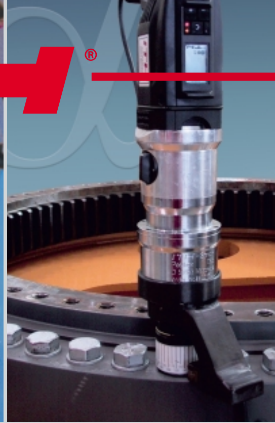
Electric rotation Nut Runner EDS-150, bolting of large roller bearing on construction machine
