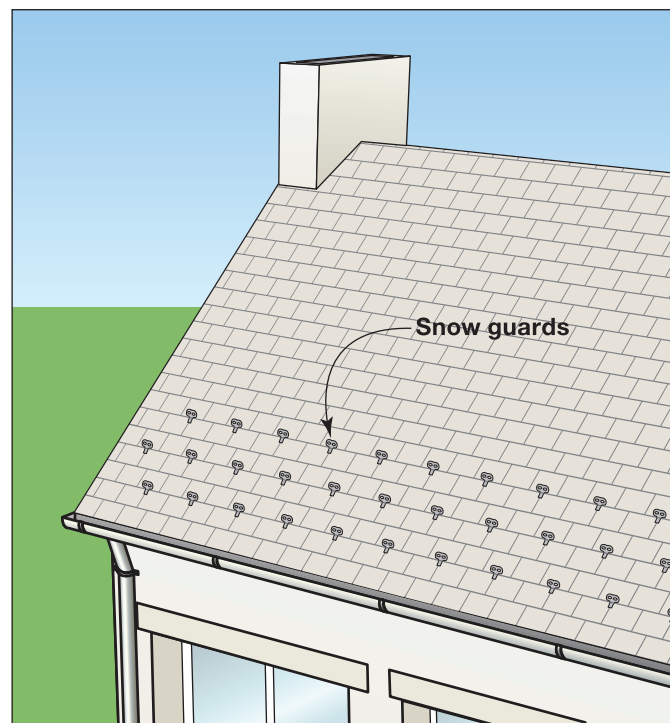
Figure 2. Snow guards or snow cleats
