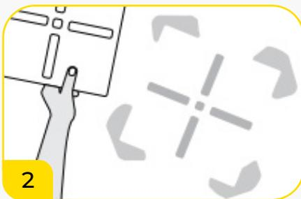
Remove AeroStencil and allow paint to dry.
