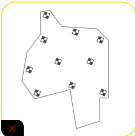
Fail: AeroPoints are missing from one part of the site (protruding area at bottom).
