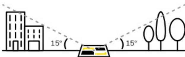
Important: AeroPoints (and/or AeroStencil marks) should have an unobstructed view of the sky in every direction above a 15° angle.
