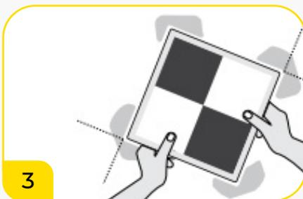
Place AeroPoint on top of AeroStencil mark, using painted corners to align exactly. Power on each AeroPoint and complete flight as usual.
