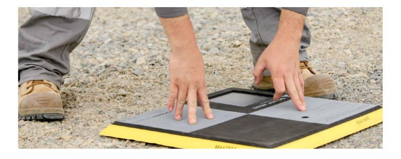
But a PPK workflow can also drastically cut down on your drone surveying setup time. All that's required for proper data capture and processing on the ground is a single AeroPoint. These robust, moveable points also function as a passive base in a PPK workflow, eliminating the need to buy an expensive base station to get your data. Using more than one AeroPoint can serve as data validation.
