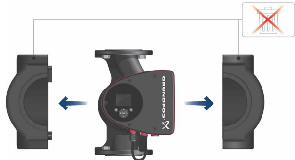
Fig. 3 Fitting insulating shells to the pump
