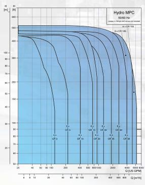
The Hydro MPC HVAC offers configurations to handle almost any head and flow, delivering consistent performance year after year.
