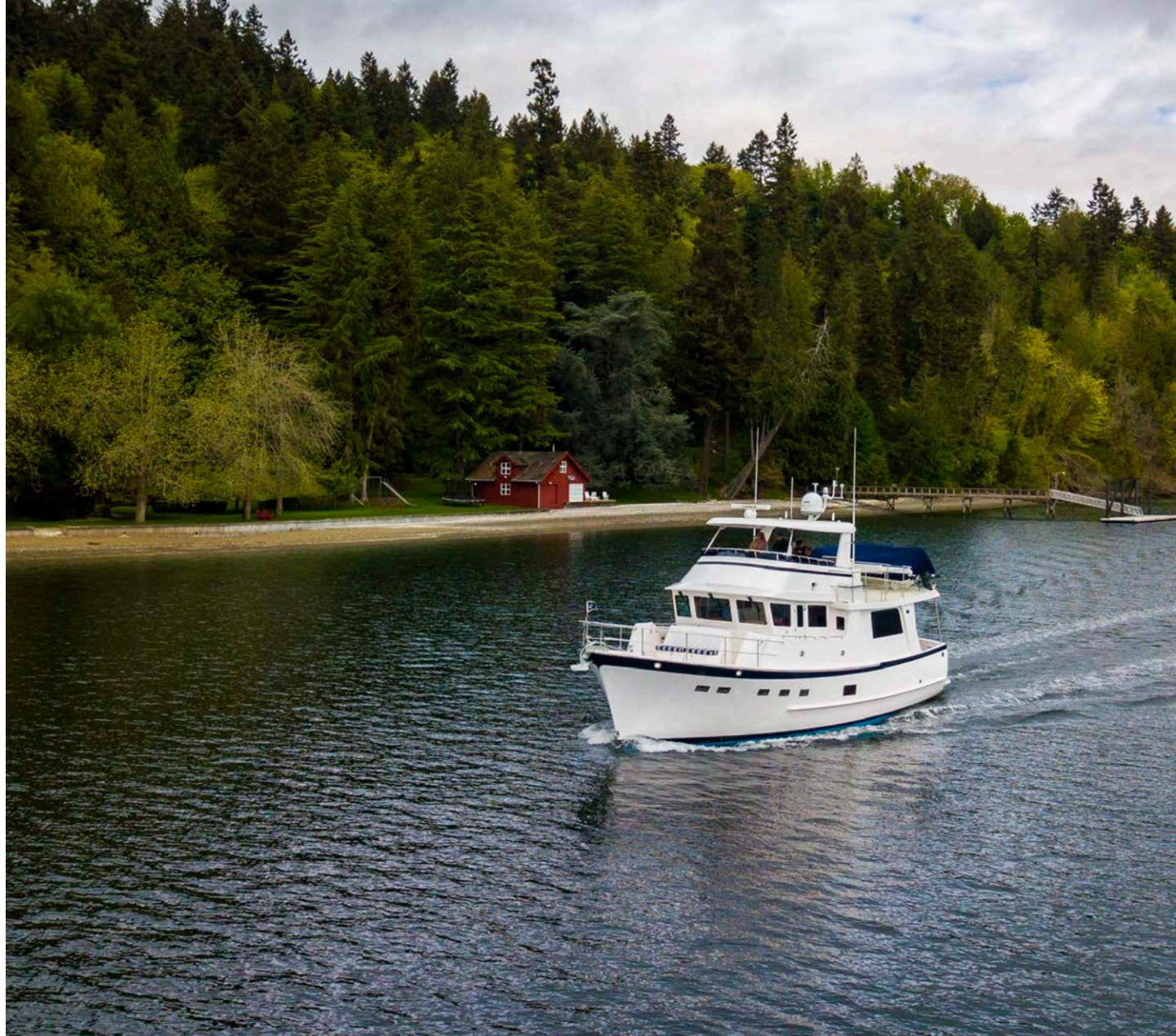
**Above:** The 50 at ease in calm seas, showing the Portuguese bridge, foredeck seating, and plentiful lights above and belowdecks. **Opposite:** The vessel features heavy stainless steel chocks and cleats and well-designed engine and thruster controls on both flanks of the pilothouse doors.
