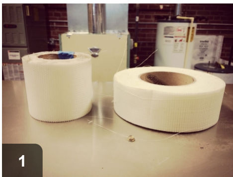
1 Use fiberglass mesh tape to cover gaps; coat with at least 2mm of mastic
