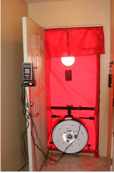
Set-up blower door to perform pressure pan testing before and after work
