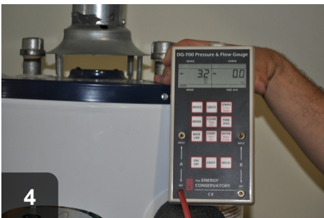
After mitigation, verify that depressurization limit is not being exceeded
