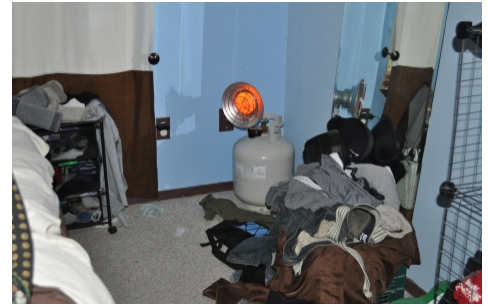
Stop the misuse of combustion appliances -- camp heater in bedroom
