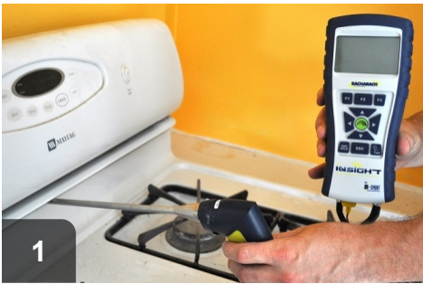
Test for CO in entire home, particularly around combustion appliances
