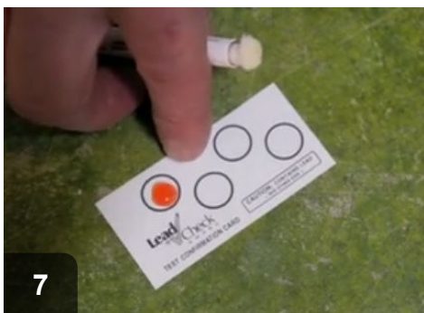
7 Lead in calibration card should test positive and turn spot red
