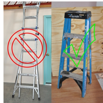
Use fiberglass ladders in place of metal
