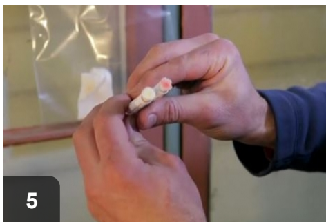
5 Red indicates lead positive. White is lead negative
