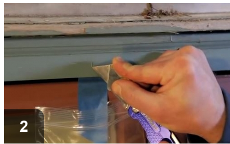
2 Place catchment bag under sample site to catch any debris. Cut sample site at an angle to expose all older paint layers
