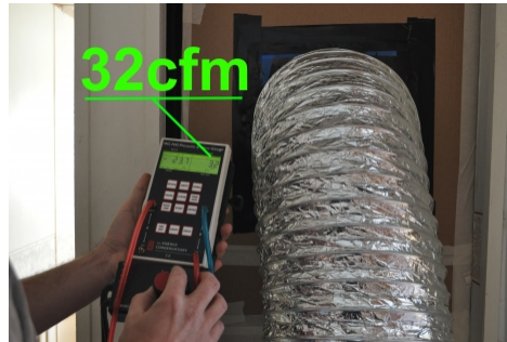
Run duct blaster test after work and compare with 'before' reading. Record result
