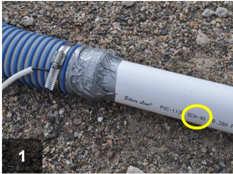
1 Select rigid fill tubes that are low conductivity -- Schedule 40 PVC fill tube
