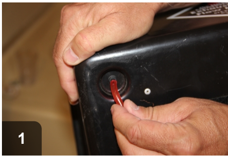
1 Attach hose to the fan meter.
