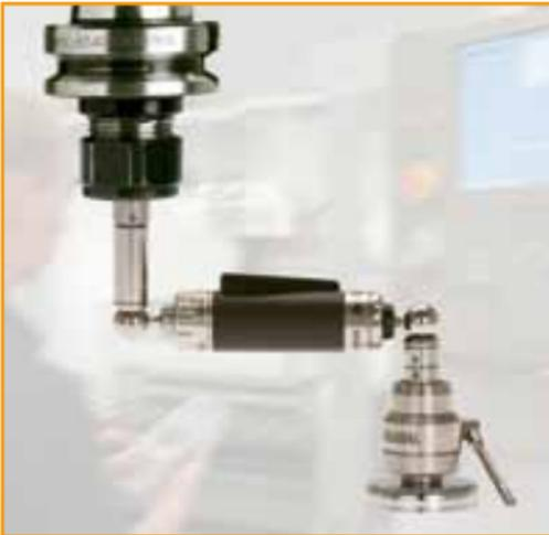
**The QC20-W ballbar system offers a fast and effective method for checking the accuracy of CNC machines. It provides comprehensive diagnosis which allows you to**
