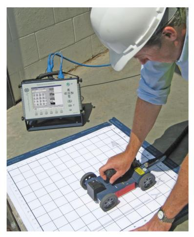
The latest Ground Penetrating Radar systems that we use are very compact, highly portable, and can access areas of a job site that X-ray cannot. Many of our clients need to drill. core or bore through slabs in out-of -the way, discrete places. Inside of a closet to run pipes through the slab seems to be a favorite, for example. Scanning and marking a clear path for these pipes can only be done with our hand-held, Palm antenna GPR systems.
