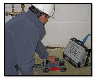
The 2.0GHz Palm Antenna is a very compact, special purpose unit. We use it for scanning in very confined spaces not accessible with the other three antennas, such as inside of closets for example.
