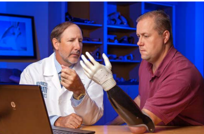
John Miguez, CP, makes final adjustments on Michael Findley's prosthesis that combines an RTV/HTV silicone liner, carbon fiber frame and Michelangelo Hand.
