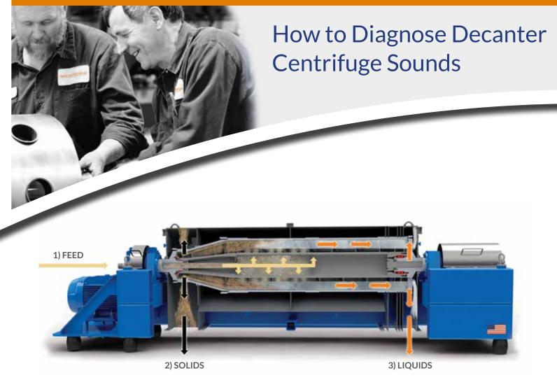
1) Feed enters the centrifuge and immediately starts spinning in the bowl. 2) The heavy solids are forced to the outermost part of the bowl and are conveyed forward through the machine with the scroll. 3) The lighter layer above solids takes the path of least resistance and flows to the liquid end of the machine.
