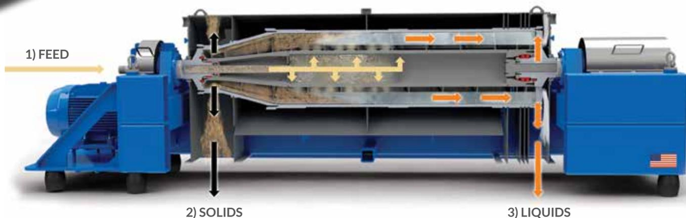
1) Feed enters the centrifuge and immediately starts spinning in the bowl. 2) The heavy solids are forced to the outermost part of the bowl and are conveyed forward through the machine with the scroll. 3) The lighter layer above solids takes the path of least resistance and flows to the liquid end of the machine.
