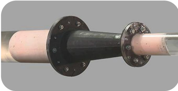
*The EVO-Pig LG is capable of reducing to half its original diameter and still remember its original size and shape.*
