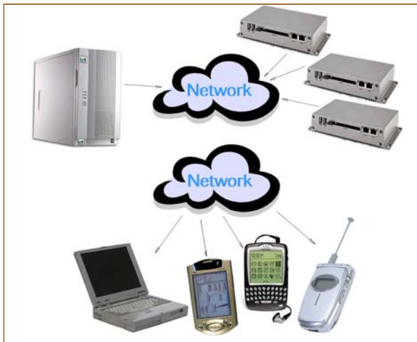
Figure 4—Example of the “Pull Strategy”. A server pulls data from the remote intelligent devices. The data is stored in a database from which it can be broadcast and made accessible via a variety of network protocols.
