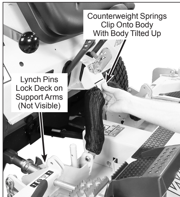
Deck Counterweight Spring Installation
