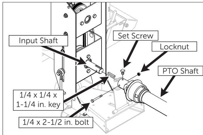
**Figure 1.1: Attach PTO Drive Shaft**
