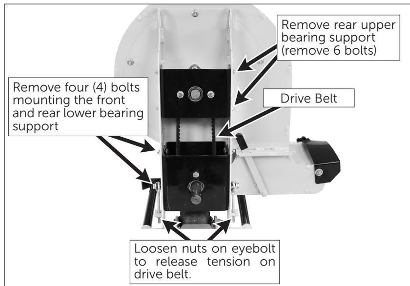
**Figure 4.1: Remove Debris Blower Drive Belt**
