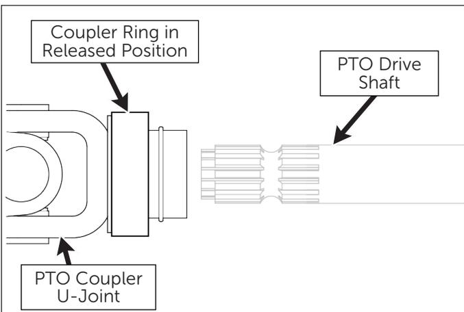
Figure 2.9: Quick Disconnect Ring in "Released" Position
