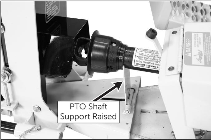
Figure 2.7: PTO Shaft Support Raised
