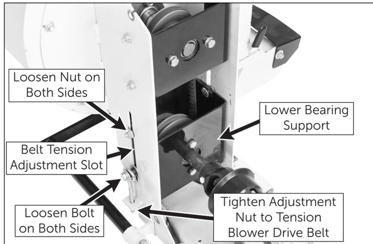
**Figure 4.3: Adjusting Belt Tension**
