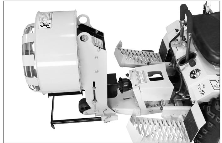
Figure 2.4: Hitch Connected to Debris Blower
