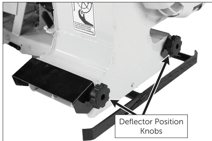
Figure 3.1: Deflector Position Knobs
