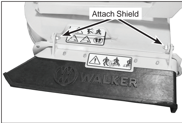
Deck Discharge Shield Installation
