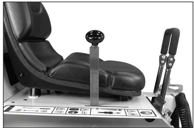
Correct FSC Lever NEUTRAL-PARK Position
