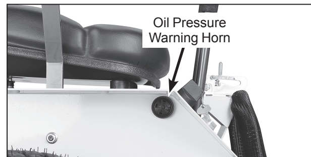
Warning Horn Location
