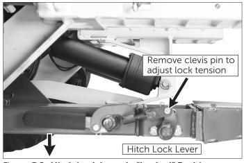
Figure 3.5 **Hitch Lock Lever in "Locked" Position**
