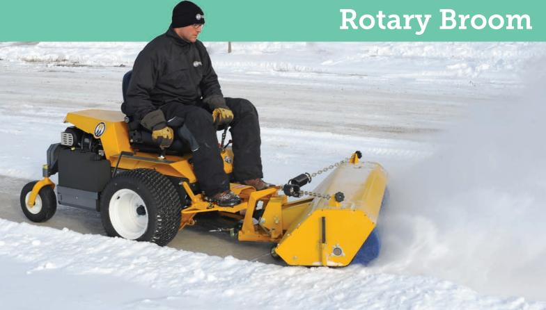
The Rotary Broom, with its large sweeping path and articulating head, is ideal for sweeping debris or light snow on hard surfaces. The Rotary Broom can also be used for lawn dethatching, raking, or sweeping gravel from turf areas.
