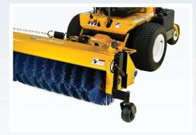
Optional Gauge Wheels are available to better control depth of brush engagement. Especially useful when working on turf. P/N I391
