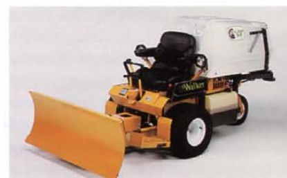
A 46-inch dozer blade, with quick-change implement hitch and power lift, is useful for moving snow, loose dirt and gravel.
