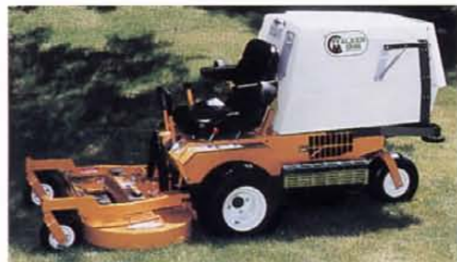
Model C — For commercial and institutional use, 16-hp Kohler engine
