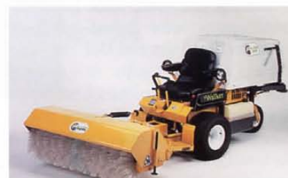
A 47-inch rotary broom uses quick-change implement hitch and power lift. Ideal for lawn dethatching, sweeping and light snow removal.
