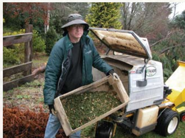
Demetri says the Walker chipper is a handy attachment that allows him to chip 80% of the gardens' branches. The hopper baskets allow him to easily spread the chips as mulch.
