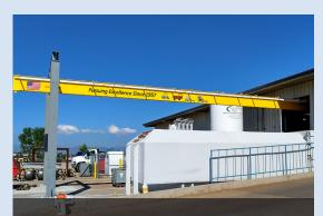
Material handling crane used to unload stacks of sheet metal from flat bed trucks and place into laser cutting storage.
