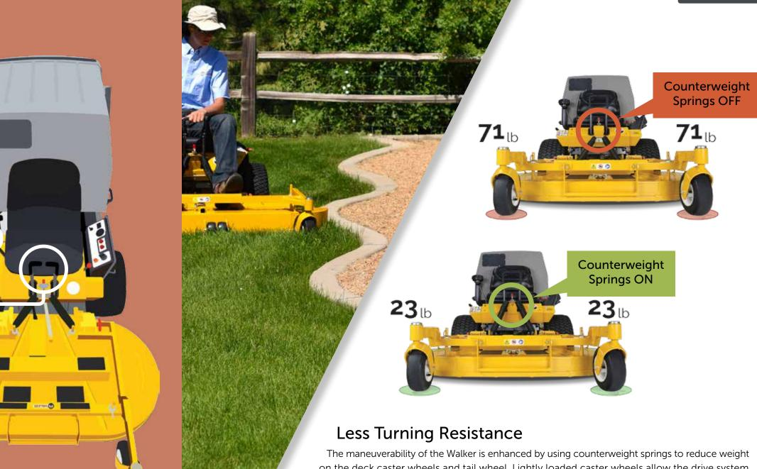
on the deck caster wheels and tail wheel. Lightly loaded caster wheels allow the drive system to immediately steer, making the Walker responsive and efficient.
