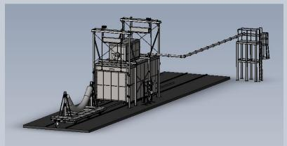
of Bends and will be installed in the new bend area of TPCN. The furnace is equipped to work with a thermal capacity of 4,000,000 BTU/hr using state of art combustion technology, including one Fives North American Burner.
