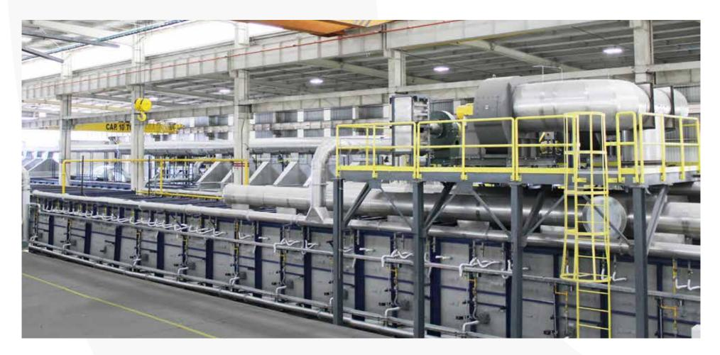
Additionally, the system employed here is capable of having different levels of internal pressure on every segment of the firing cycle. The pressure is monitored constantly by the system and controlled by the ceramic louver type damper.
