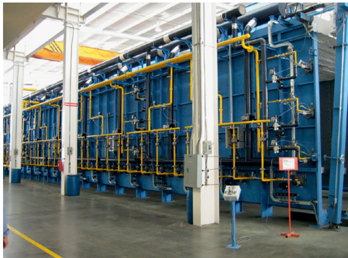
Fig. 3 IMPS® shuttle kiln for vitrified clay pipes
