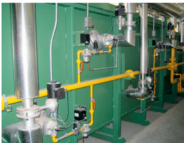
Fig. 4 IMPS® tunnel kiln for technical ceramics using pre-heated combustion air
