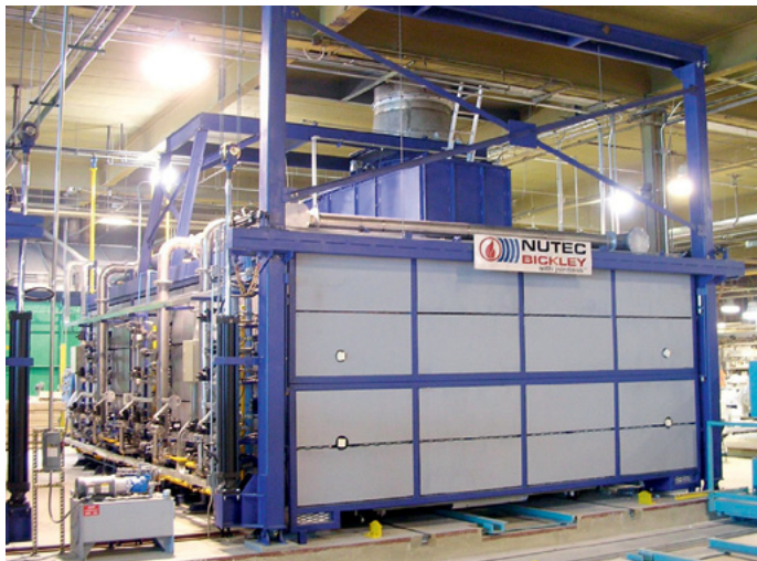
Fig. 2 IMPS® shuttle kiln for sanitaryware
