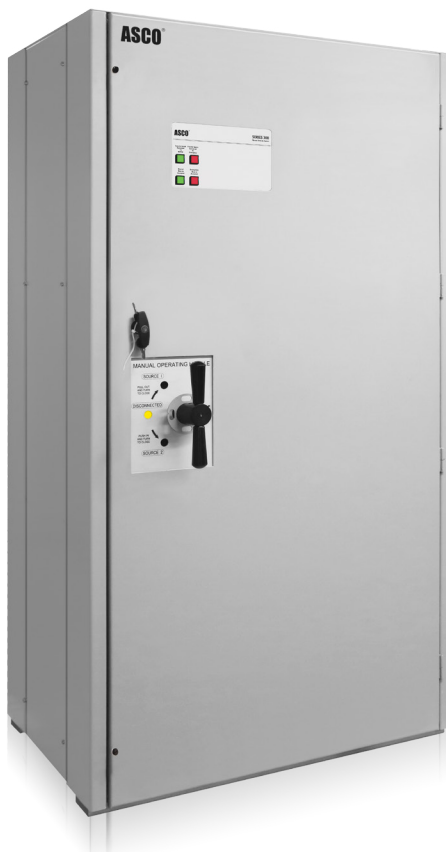
Figure 3: Three-position switches allow motors to slow before loads are transferred to an alternate power source. This helps avoid excessive inrush currents.
