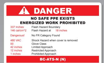
REMEMBER: an ARC FLASH HAZARD ANALYSIS must be performed by an independent expert in order to provide the appropriate information needed by a trained technician to determine the correct safety processes and PPE needed to inspect and maintain that switchgear.
