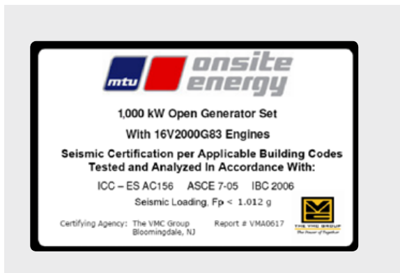
Figure 4. A typical label on a seismically certified generator set referencing the applicable IBC version and the upper seismic loading limit, FP.
