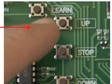
3. Press **Down**: Move door to required **closed** position—press **learn** to confirm position and commence automatic check of both settings
