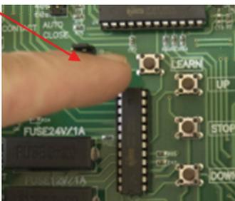
2. Press **Up**: Move door to required **open** position—press **learn** to confirm position and commence learning of closed position
