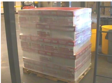
Example of a correctly stacked and stretch-wrapped pallet
