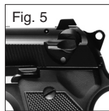
Mod. G Decocking lever only - Return to the ready to fire position
