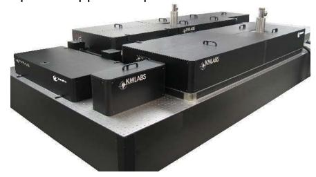
Red Dragon<sup>™</sup> is KMLabs' multi-stage multipass amplifier providing high-energy sub-25 fs pulses. It is a fully engineered and integrated commercial source based on a single rugged opto-mechanical platform. It employs patented (US 6,804,287) cryogenically-cooled amplifier technology, allowing for continuous trade-off between pulse energy and repetition rate.
