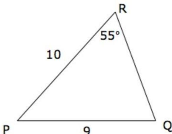
When given two sides and a non-included angle, write down the sine rule.
