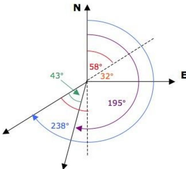
The third angle in the triangle =  $180^\circ - 43^\circ - 32^\circ = 105^\circ$
