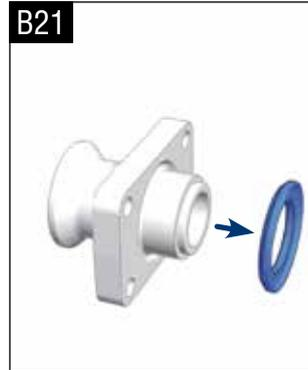
Dismantling of bearing bushing /rod guidance system (1 & 2)
