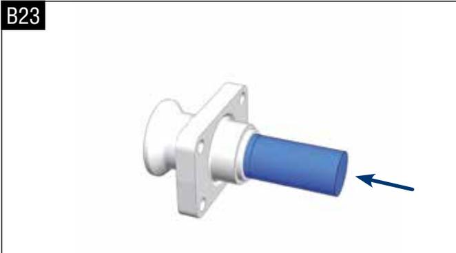
Dismantling of bearing bushing /rod guidance system (3)
