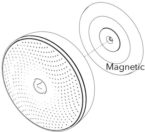
Fix the mounting bracket to the ceiling or wall. Make sure you use appropriate screws for your wall type. The screws included are intended for wood or drywall. Do not place it close to vents or windows. Minimum 1 meter / 3 feet distance.
