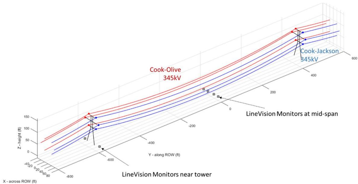
Figure 6: Orthographic Projection View. Gray boxes represent EMF monitors.
