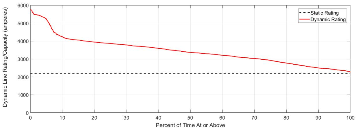
Figure 10: Histogram for the month of January 2017, showing the amount of time the line's capacity was at, or above, its Static Line Rating.
