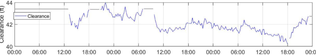
Figure 7: Conductor clearance in feet over a 3 day period.
