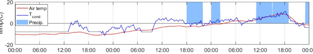
Figure 8: Conductor temperature and ambient temperature in Deg C over a 3 day period.
