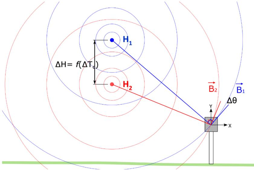
Figure 1 (Left): EMF monitor detecting the angular change of the EMF signal, as a single conductor sags from  $H_1$  to the lower position  $H_2$  when it is heated.
