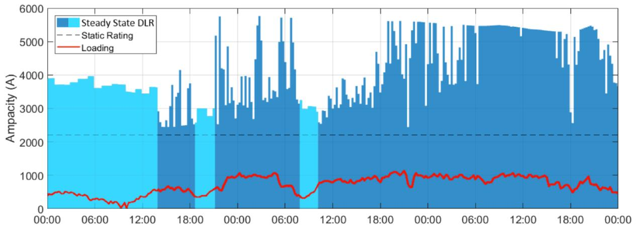
Figure 9: Circuit loading, Steady-State DLR, and Static Line Rating (SLR) shown over a 3 day period. The lighter shade of blue (teal) indicates times when the system utilized the external weather data source as opposed to the sag as determined from the LineVision EMF monitors.
