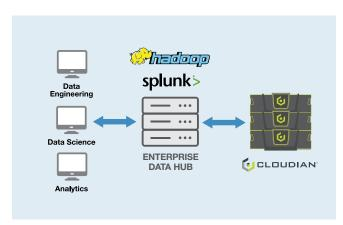
data backup target or as an active archive tier for analytics workloads. Splunk SmartStore enables native S3 connectivity with Cloudian, decoupling the compute needs from storage requirements and reducing the overall TCO by more than 60%.
