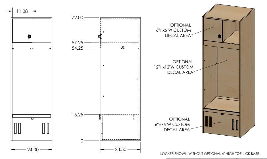
OPEN FRONT LOCKER, 24"W x 24"D x 72"H (NOT INCLUDING OPTIONAL BASE) \* 3/4" MAPLE VENEER PLYWOOD WITH 3MM WOOD EDGE BAND; SOLID HARDWOOD TRIM; GLUE AND DOWEL CONSTRUCTION \* INCLUDES BUILT IN COMBINATION LOCK ON UPPER CUBBY, FOOT LOCKER LIFT LID WITH HASP LOCK, 3 DOUBLE HOOKS, VERTICAL VENT SLOTS ON LOWER FOOT LOCKER FACE (BLACK COLOR) ALL HARDWARE IS SILVER COLOR
