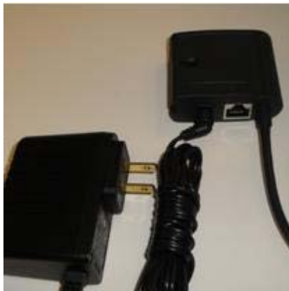
Connection of power supply for a serial link to Point-of-sale System
